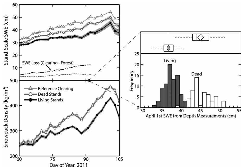
**Figure 3** | Stand-scale SWE and snowpack density graphed against Day of Year, 2011. Dot markers in SWE and density graphs represent average measurements, and shaded regions represent 95% confidence intervals. *SWE Loss* in the stand-scale SWE graph was calculated as reference clearing SWE minus forest SWE. A histogram of snow depth values in living and dead forest stands for 1 April with average, maximum, median, minimum and quartile distribution values is inset.
